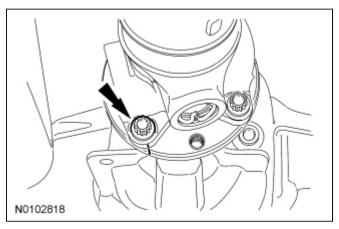
4. **NOTE:** The driveshaft flanges fit tightly on the flange pilots. Never hammer on the driveshaft or any of its components to disconnect the driveshaft flanges from the flange pilots. Pry only in the area shown, with a suitable tool, to disconnect the driveshaft flanges from the flange pilots.
