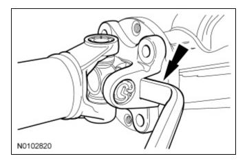
5. **NOTE:** The driveshaft flanges fit tightly on the pinion flange pilots. To make sure that the driveshaft flanges seat squarely on the pinion flange pilots, tighten the driveshaft flange bolts evenly in a cross pattern.
